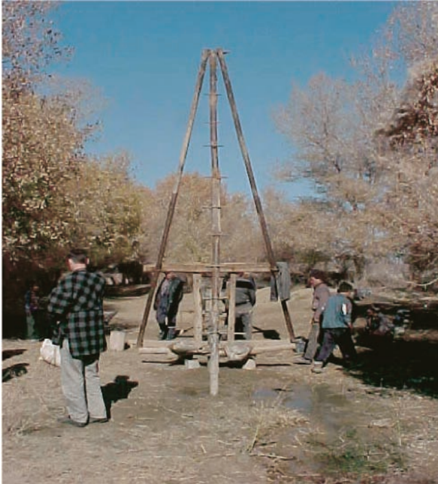
Hand-operated, cable-tool drill rig.
