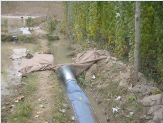
**Picture 7: Inline tarp intake: excess water is from previous tests; there is no leakage here**
